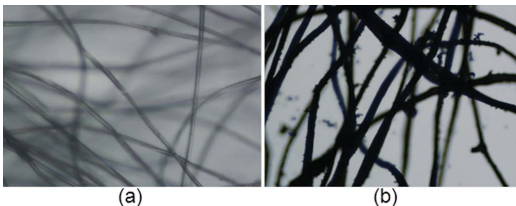
Figure 7. Optical microscopic images of (a) untreated silk and (b) PPy-coated silk [ \times 20 magnification]. [Color figure can be viewed in the online issue, which is available at wileyonlinelibrary.com.]
